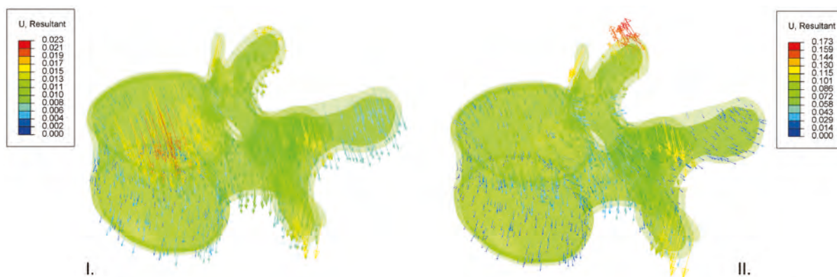
FIGURE 14 | THE DISPLACEMENT CAUSED BY THE LOADING CONDITION IS ILLUSTRATED USING VECTOR FIELDS. THE FIGURE DEPICTS THE SAME RESULT AS FIGURE 13B, BUT IT USES ANOTHER GRAPHICAL APPROACH. ONE OF THE KEY BENEFITS OF FEA IS THAT THE USER CAN CHOOSE BETWEEN THE DIFFERENT RESULT VISUALIZATION OPTIONS
